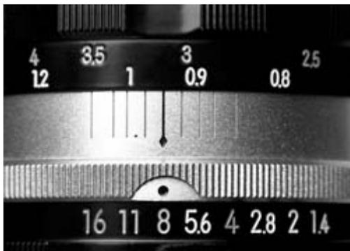
the aperture settings on a lens corresponds to how wide the lens opens when a picture is taken.
